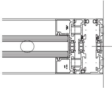
STANDARD PANEL-TO-PANEL CONNECTION WITH GASKETS
